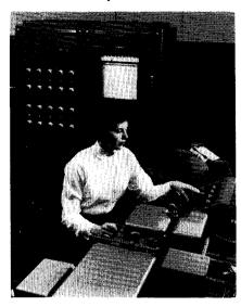
Automatic analyzer in operation. Operator selects ten different analytical wave lengths by means of the potentiometers mounted on the master control panel. The selected wave lengths are then fed into the control unit, which controls operation of the instrument for the analysis
